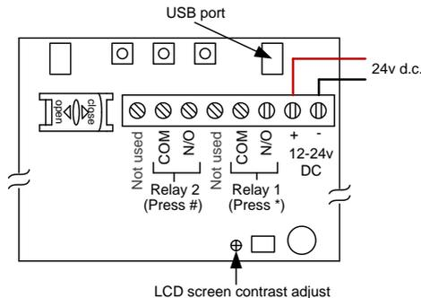
**WARNING:** Current draw when in operation spikes at up to 2 amps. Do not use alarm cable or CAT5 cable to connect power to this device.
