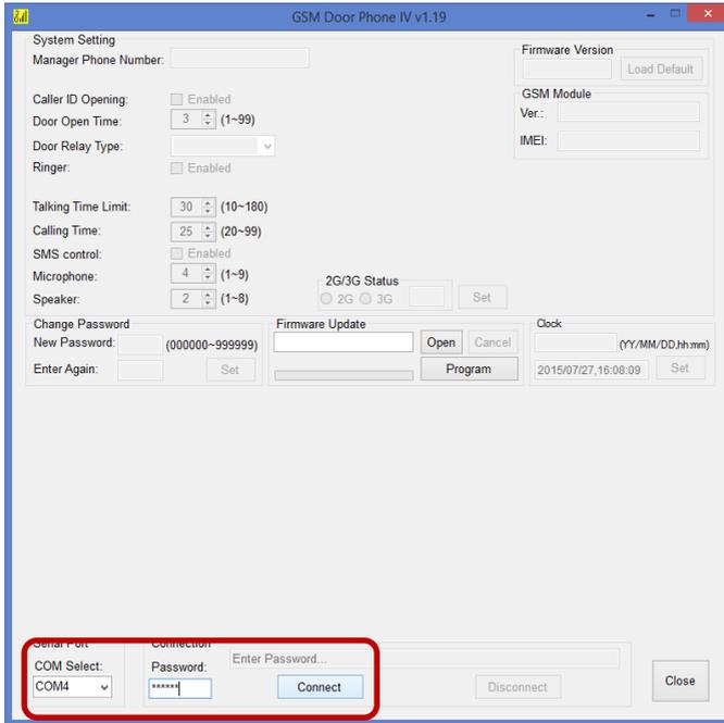
The window above will appear. Select each COM port option shown bottom right until an error message does not appear (this will indicate the correct USB COM port has been selected). Then enter the manager password (default 123456) and press CONNECT.
